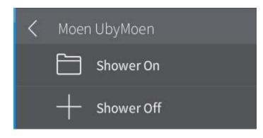
**Shower On** – this is selected to cycle an outlet from off to on. The installer settings Cycle Seconds defines the time between on and off.
