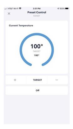
The left screen shot allows the end user to manually select a preset to be turned on. If a preset has been selected, the right screen shot shows how to control the preset. Tapping the "+" or "-" buttons will increment/decrement the temperature set point. Tapping "off" will turn the shower off.
