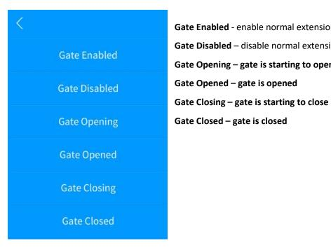
**Gate Enabled** - enable normal extension functions **Gate Disabled** – disable normal extension functions Gate Opening – gate is starting to open Gate Opened – gate is opened
