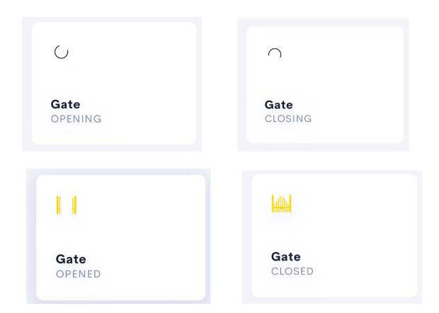
The above 4 images show the feedback as the gate goes from being opened, closed, opening, and closing. Opening and closing states will show a spinning circle for the number of seconds defined in the installer options.
