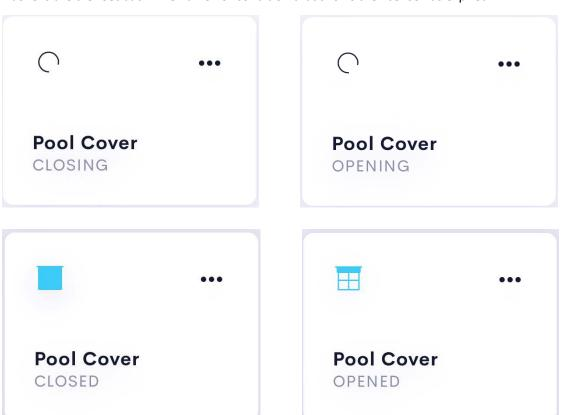
The above 4 tiles show status feedback as the pool cover moves from closing, to closed, opening, to opened.
